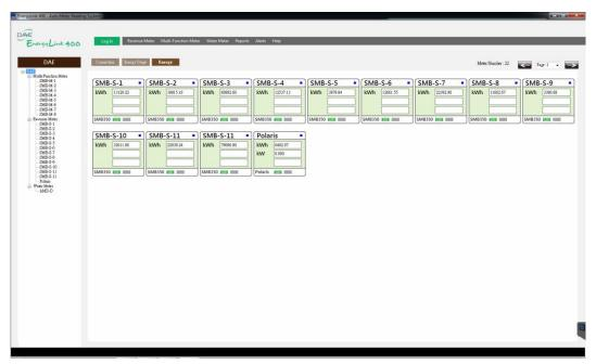
The left side of the screen shows an outline of the current layout of the building or campus, which is prearranged according to the preference of the facility manager by building, floor or zone for ease of finding the desired meter.
