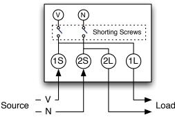
**Note**: Always make sure that shorting screws are tight when in normal use, shorting screws are loosened only during testing and calibration.
